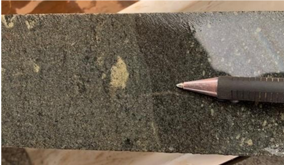
Figure 7-5 Example of sharp contact between two diorite bodies
