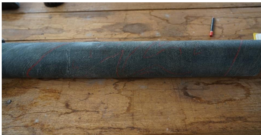
Example of buckle folds within the diorite. MRRD007, 154.06m. Source: Montage
